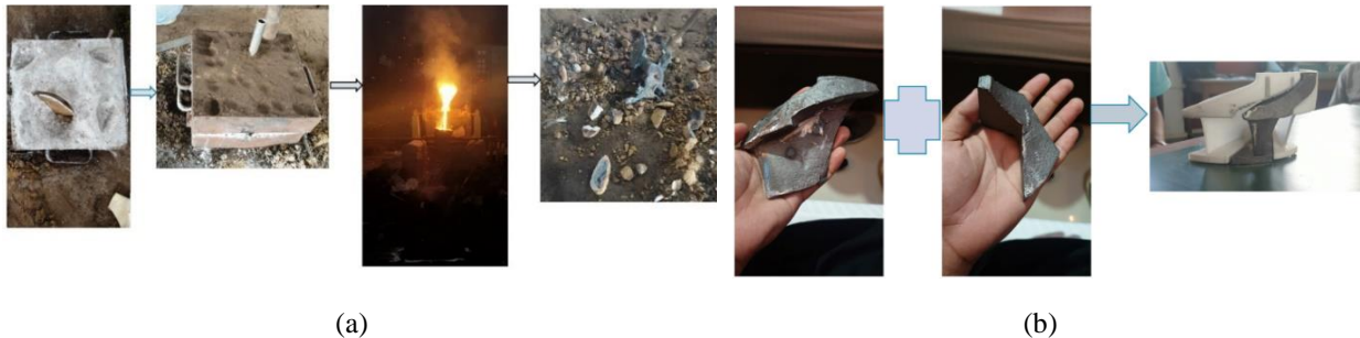
FIGURE 5. (A) Sand Casting Process at Metal Cast FIGURE 5. (B) Finished Product (Casted Section of Francis Turbine Runner)
