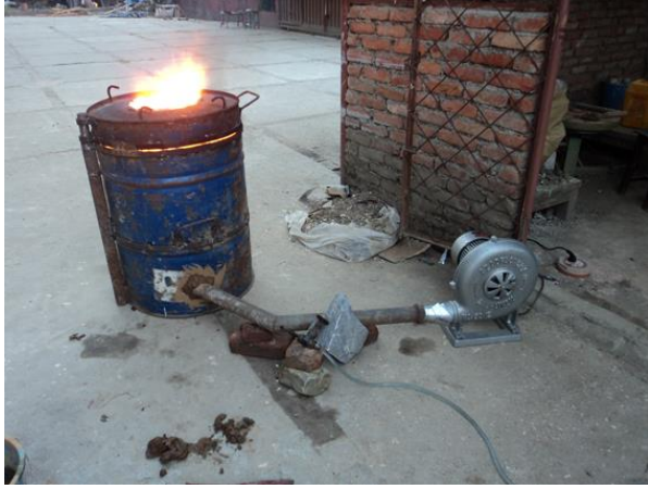
Fig. 27 Locally improved home based multi-fuel furnace by Tejesh Man Shakya in 2006 A.D. for metal melting
