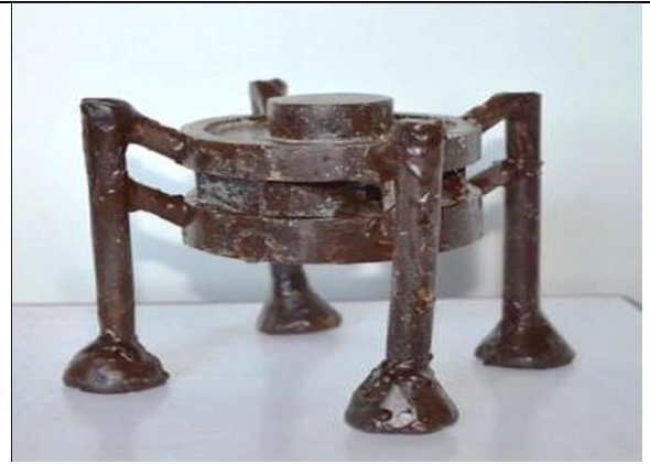
Fig. 24 Wax Francis Runner with added Sprues and Vents
