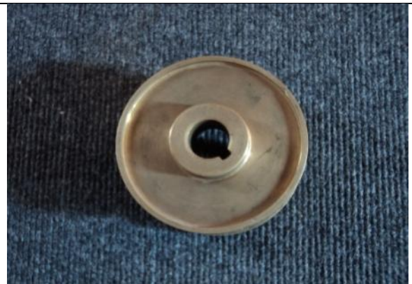
Fig. 32 Final fabricated cast brass Francis Runner after chasing and finishing
