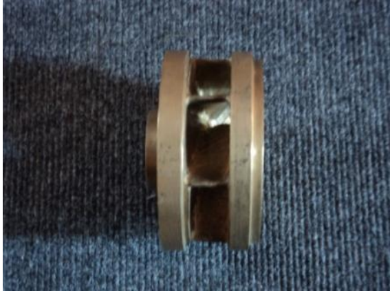
Fig. 33 Final fabricated cast brass Francis Runner after chasing and finishing
