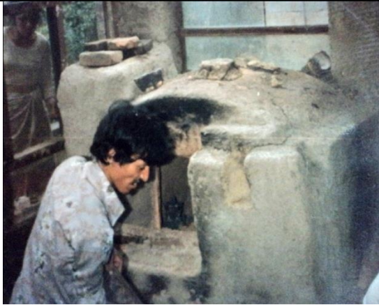
Fig. 35 Locally improved Petroleum Kiln with Traditional Materials for Mould Baking by Tej Ratna Shakya in collaboration of Mechanical Engineer Nira Prasad Hyoju at Foundry of Gharelu Moortikala Udyog 1986 A.D.
