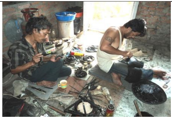
Fig. 12 Home based traditional wax modeling process
