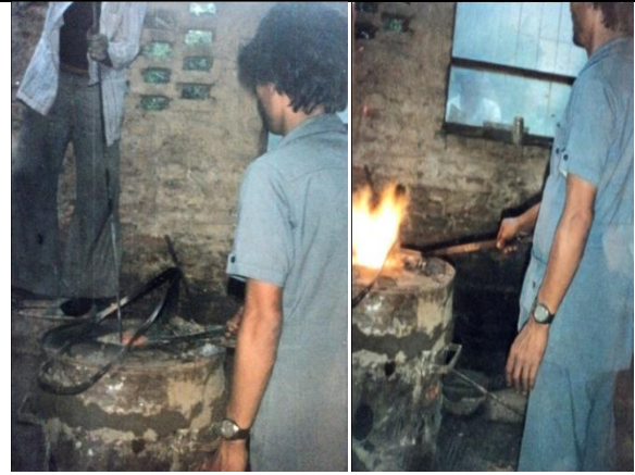
Fig. 36 Locally improved Petroleum Furnace for Melting Metal by Tej Ratna Shakya in collaboration of Mechanical Engineer Nira Prasad Hyoju at Foundry of Gharelu Moortikala Udyog 1986 A.D.
