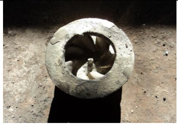
Fig. 30 After cutting sprues and vents of cast brass Francis Runner
