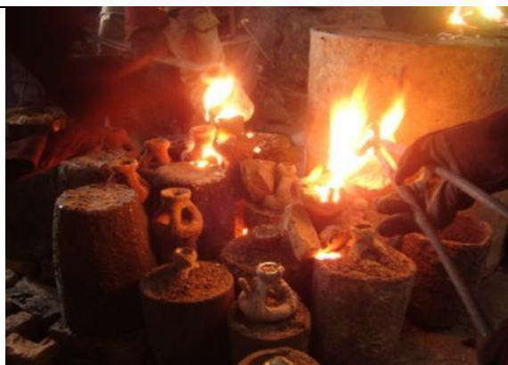
Fig. 17 Pouring molten metal into the traditional mold
