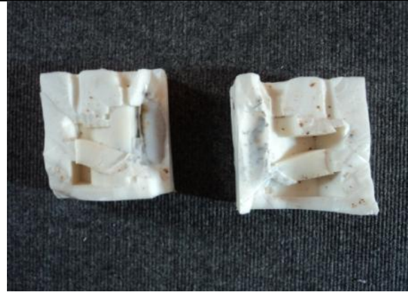
Fig. 22 Silicone Rubber Mould of Section of Francis Runner
