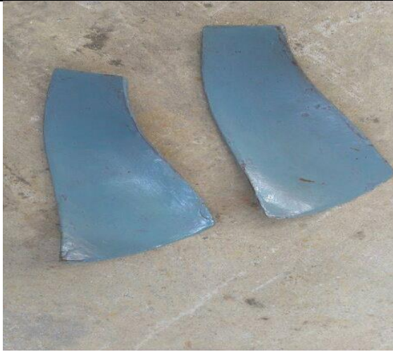
Fig. 19 Francis Blade Model casted in Dhalot Karyashala (Sand Casting Technique)
