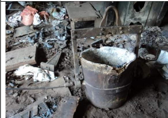
Fig. 3 Crucible for melting Metals at Dhalaut Karyashala
