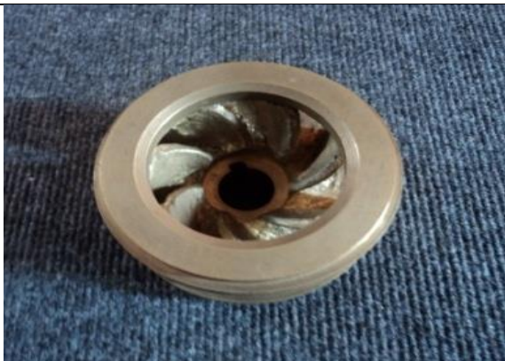
Fig. 31 Final fabricated cast brass Francis Runner after chasing and finishing
