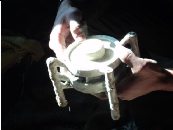
Fig. 29 After break open gypsum based mould of Francis Runner
