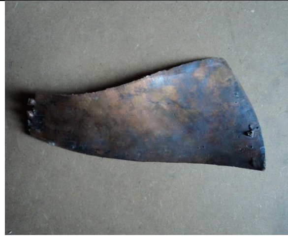
Fig. 20 Francis Blade Model casted in Durga Handicraft (Vacuum Casting Technique)
