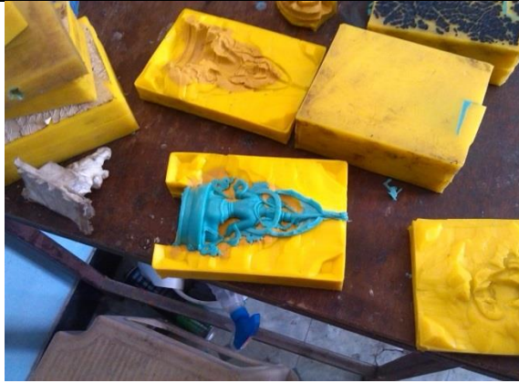
Fig. 7 Silicone Rubber Mold for Wax Casting
