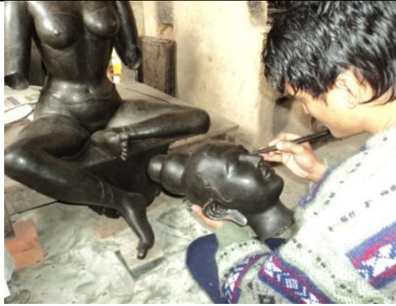
Fig. 13 Home based traditional wax modeling Process
