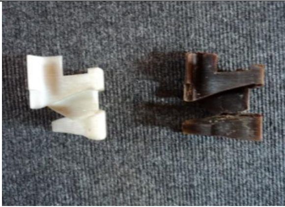
Fig. 23 Cast piece of wax (Right) from Silicone Rubber Mould of Section of Francis Runner
