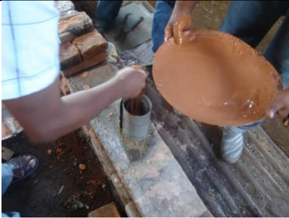
Fig. 37 Preparing Gypsum based Mould - 1 st locally organized workshop on Italian Lost Wax Casting Method at Foundry of Ethnic Fine Art November 2006
