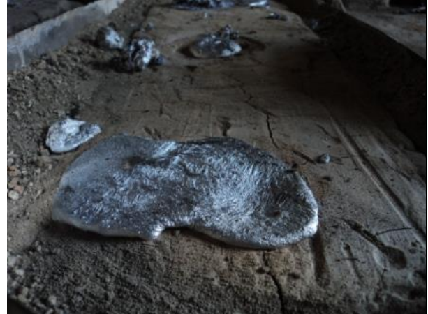
Fig. 28 After pouring the brass into the gypsum based mould of Francis Runner
