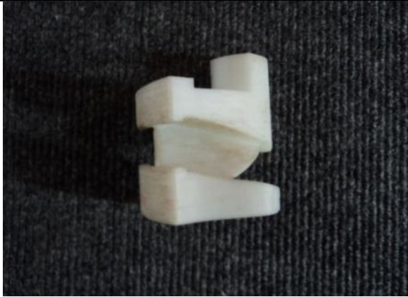
Fig. 21 Section of Francis Runner developed from Rapid Prototype Machine
