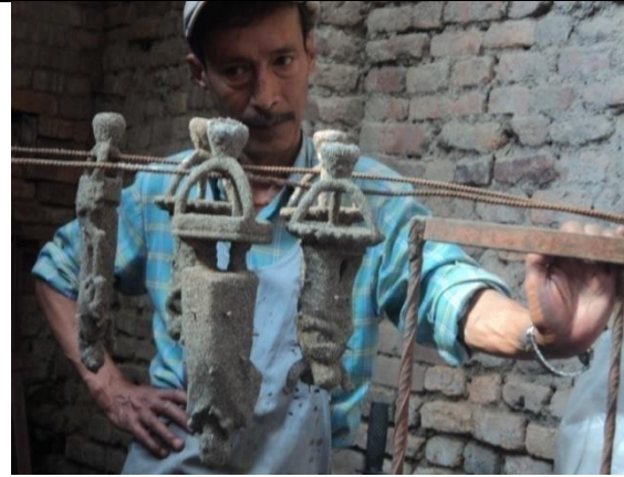
Fig. 38 Ceramic Shell Mould for Lost Wax Casting Process - Locally experimented Foreign Foundry Technology at Foundry of Ethnic works Art & Design January 2012
