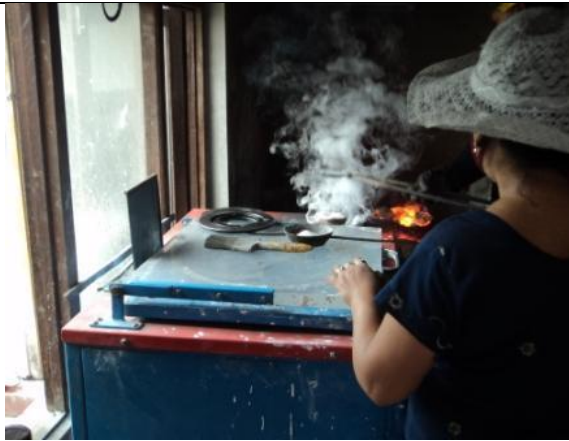
Fig. 9 Pouring molten metal into the Mold inside Suction Machine for Vacuum Casting
