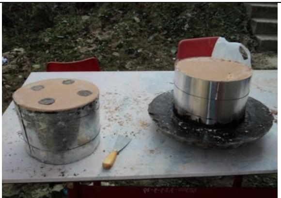
Fig. 25 Casting Mould of Francis Runner prepared from slurry of gypsum based powder for Italian Lost wax casting
