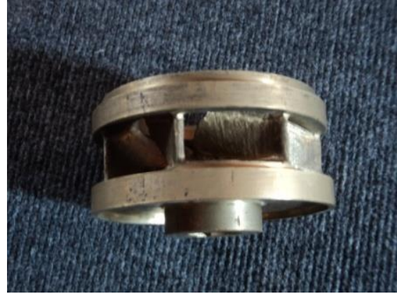
Fig. 34 Final fabricated cast brass Francis Runner after chasing and finishing
