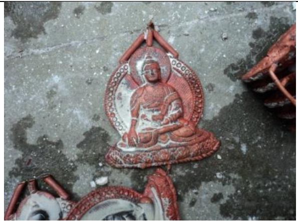
Fig. 10 Copper image of Buddha from Vacuum Casting Process
