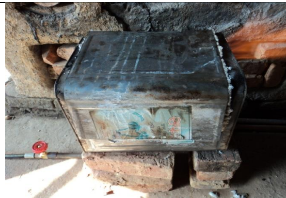
Fig. 26 Locally improved home based gas kiln by Tejesh Man Shakya in 2006 A.D. for mould baking
